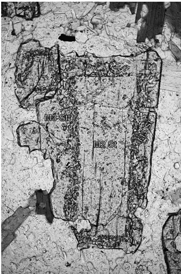
Fig. 11. Late-stage overgrowth of M3 St on M2 crystallite from the partial pseudomorph shown in Fig. 10. Plane polarized light. Long dimension of field 1.6 mm.
