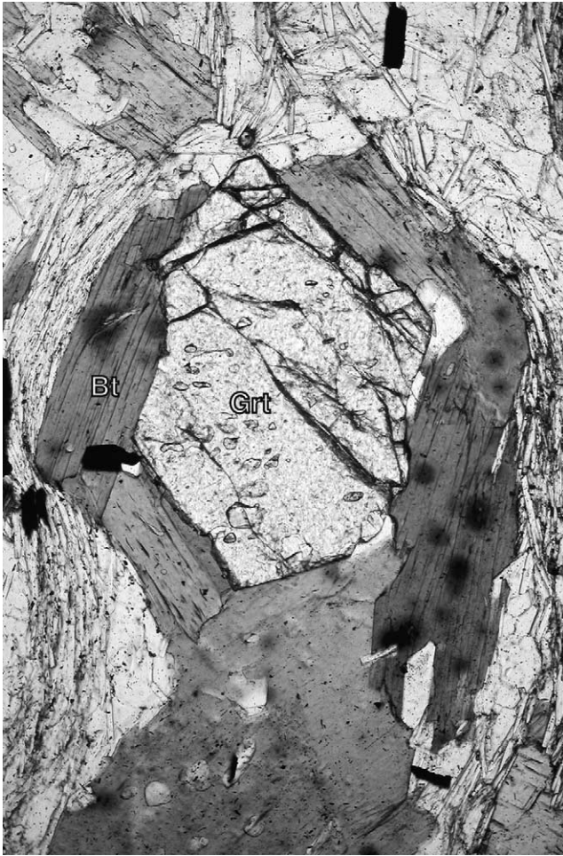
Fig. 17. Coarse Bt rims around Grt from M3 LSZ. Bt laths surrounding Grt core preferentially grew parallel to Grt crystal faces. Plane polarized light. Long dimension of field 1.5 mm.
